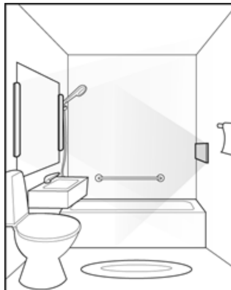
Figure 1. Experimental setup of bathroom: Two lighting fixtures by the bathroom mirror for main and task lighting, and one fixture above the bathtub for shower and bath lighting.
