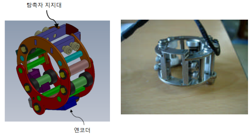
Fig. 7 Hand driving manual encoded scanner for small bore socket weld piping
