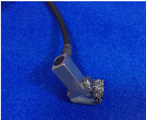
Fig. 12 Manufactured phased array ultrasonic transducer and wedge
