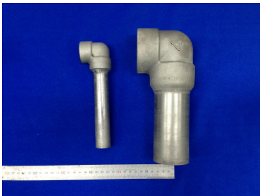
Fig. 10 Photo of manufactured flawed socket weld specimens
