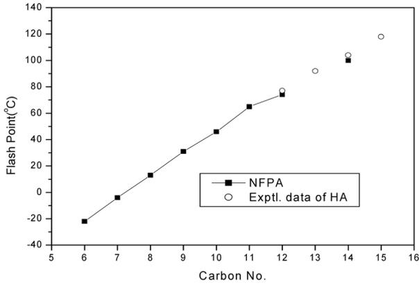
Fig. 1. A comparison between NFPA and Ha' flash points for n-alkanes.
