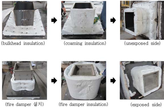
Figure 5: Process of specimen production.
