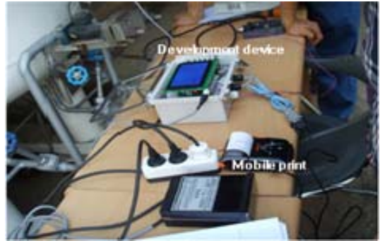
Figure 8: Overview of test for the developed digital level meter
