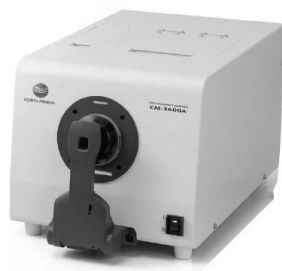
Fig. 2. Spectrophotometer (CM-3600A, Konica Minolta, Tokyo, Japan)
