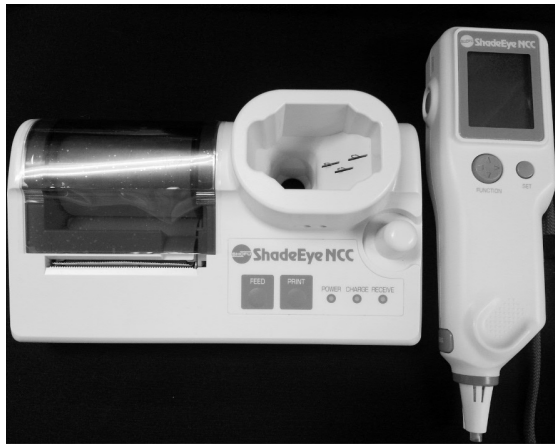
Fig. 2. ShadeEye-NCC® dental chromameter (Shofu Dental, Kyoto, Japan)
