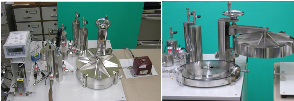
Figure 2. Gas pycnometer system (left: a photograph of the whole unit, right: Detailed view of the sample chamber).
