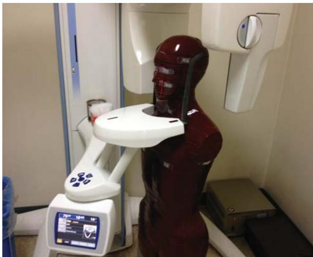
**Fig. 1.** The limbless female whole body phantom.
