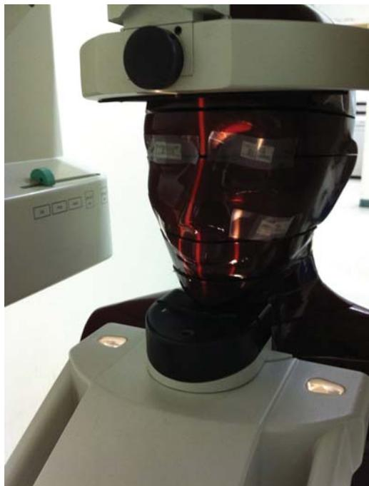
**Fig. 2.** The head phantom representing a man.
