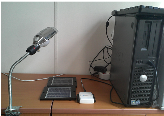
Fig. 3 A fault detection test-bed of the photovoltaic system
