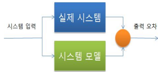
Fig. 1 A schematic diagram of fault detection system
