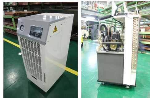
Fig. 2 The appearance and inner picture of industrial cooler of on-off control method
