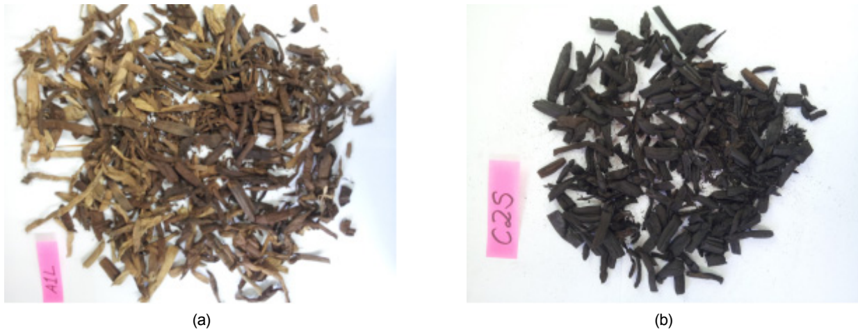
Figure 4. Color change of samples at different temperature: (a) 200°C, (b) 300°C.
