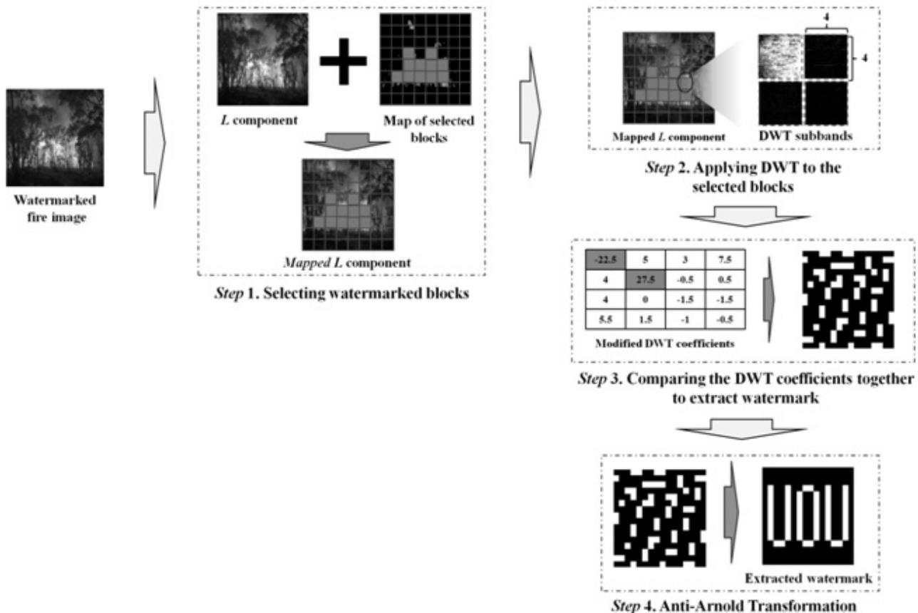
Fig. 4. Watermark extracting process of the proposed approach
