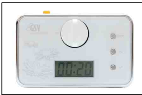
Fig 1. Gas valve time control system
