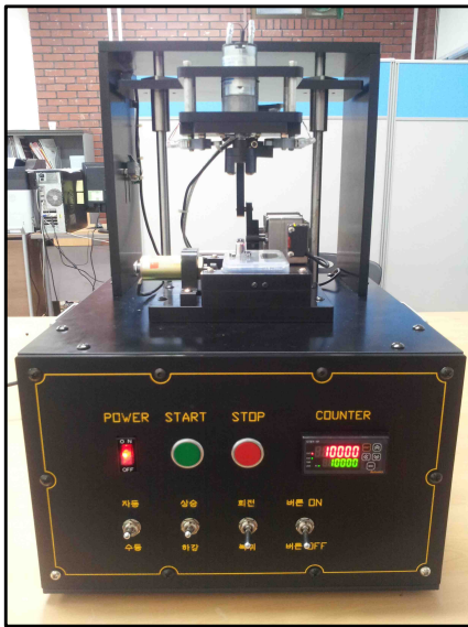
Fig 8. Gas valve control repeat check system
