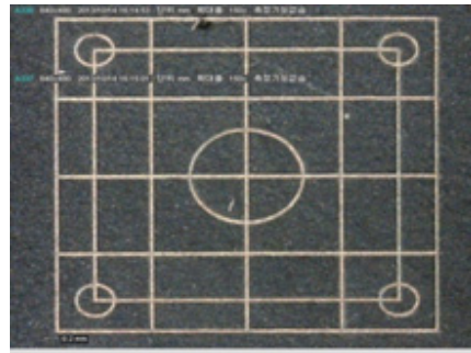
Fig. 6 Engraved patterns in the printing roll of 10mm × 10mm area.
