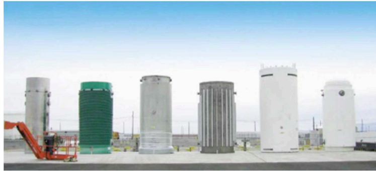
Fig. 3. NAC-128, CASTOR V/21, REA 2023, MC-10, VSC-17, and TN-24P Dry Storage Casks used for the Storage Demonstration Project at the Idaho National Laboratory [4]
