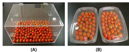
Fig. 1. The pictures of 50 mm acrylic container(400×250×200 mm) for  $\text{ClO}_2$  gas pre-treatment (A) and PET container(265×205×55 mm) for storage (B).
