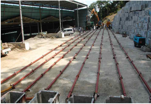
Figure 1. Horizontal pumping test
