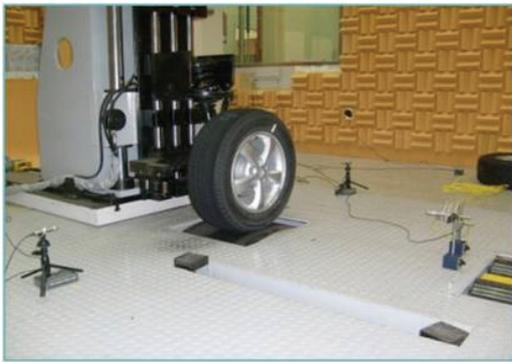
**Fig. 5** Photograph of actual tire noise measurement
