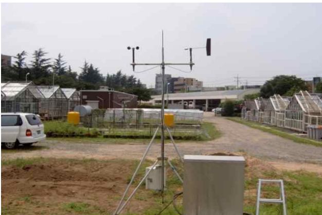
Figure 4. Wind speed and direction measured for the drift control test.
