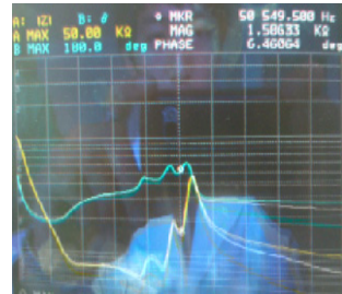
[Fig. 10] Result of M-layer(OD: ϕ62mm.T: 12mm)
