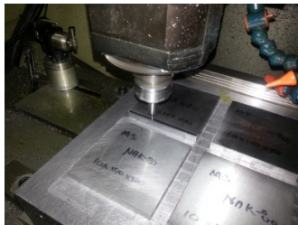
(a) Installation of tool dynamometer and material processing
