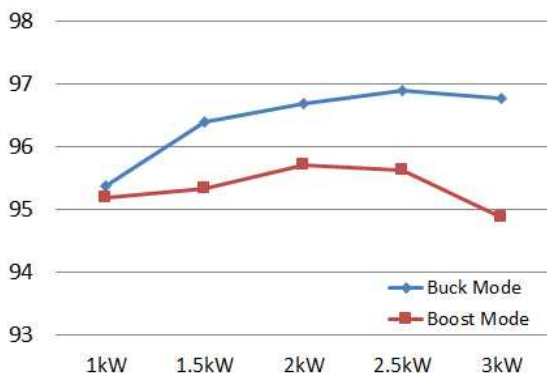
Fig. 15 Measured efficiency as a function of the output power at V_L = 80V using Yokogawa WT3000
