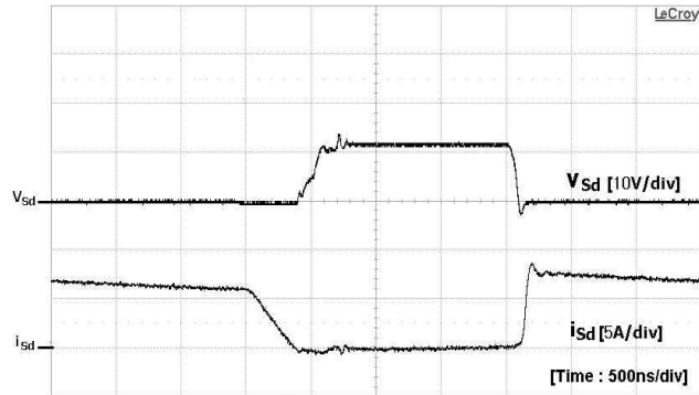
Fig. 8 Experimental results of synchronous switch S_d
