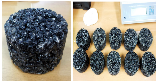
Fig. 2 Porous Asphalt Concrete Pavement Specimens
