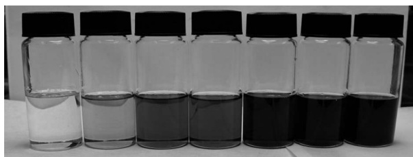
Fig. 2. Image of the oxidized soybean oil samples, from the left: virgin oil, 0.33, 1.19, 1.75, 2.38, 3.03, 3.67 mg KOH/g.
