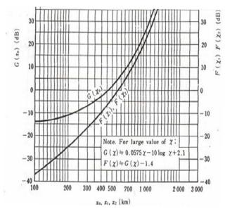
Fig. 2. The Alternative Solution Sheet for Additional Loss(Shibuya, 1987).
