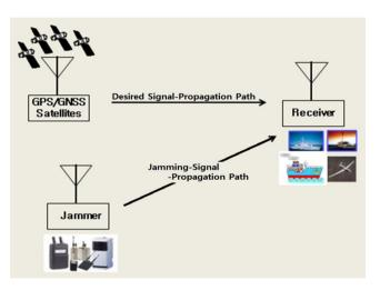
Fig. 1. The concept of GNSS Jamming.
