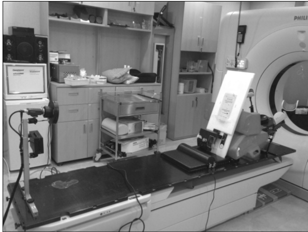
Fig. 4. The motion of the respiratory Gating Platform (RGP) was measured by using the RPM system, independently.
