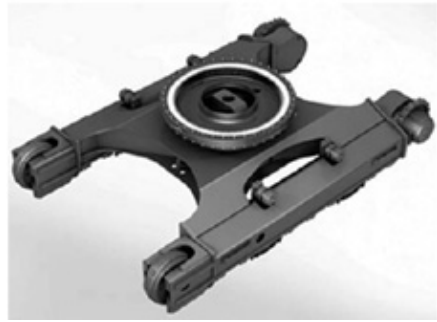
Fig. 1. Example of lower center frame of excavator
