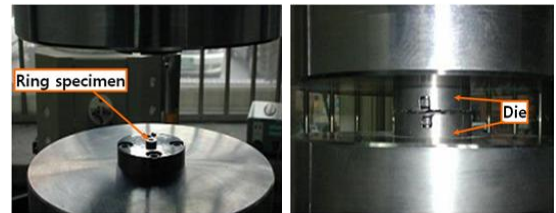
Fig. 3 Ring compression test
