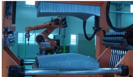
Fig. 9 Flexible stretch forming apparatus
