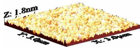
Fig.1. Image AFM of p-type Si (100) wafer after cleaned.
