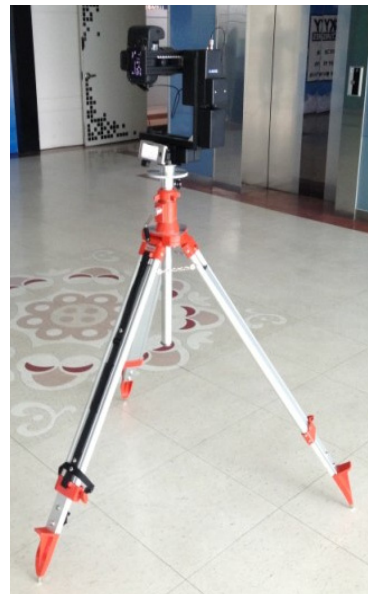
Figure 2. Non-metric Camera Module with Motorized Head
