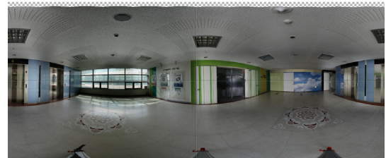
Figure 4. Good Case of Image Stitching(35mm Lens, V5(33.82%), H12(20.63%))
