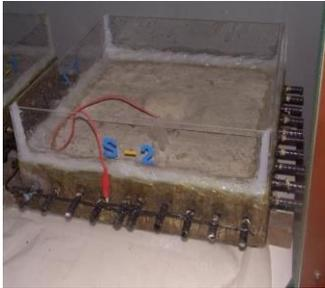
Fig. 3 Specimen after anode was installed
