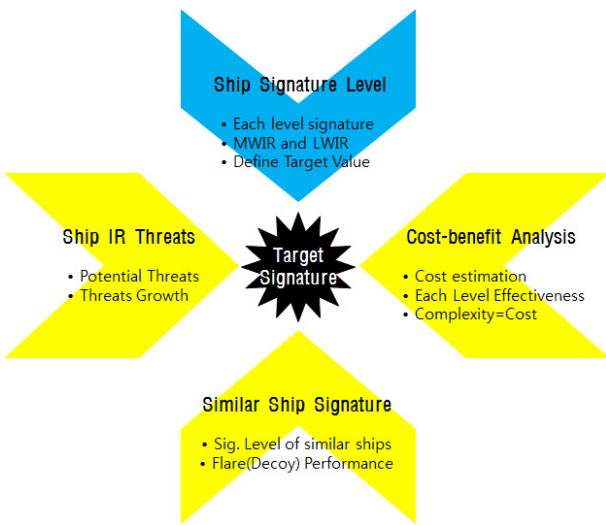
Fig. 8 Decision-making of ship signature target (criteria) by considering the design parameters
