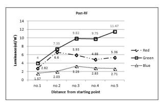
Figure 11. Effect of the luminance values by the color of light source in the condition of Post-RF(unit:  $cd/m^2$ ) Post-RF(Post-etching × Reflective Fabric)
