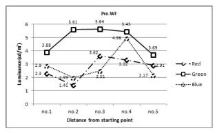
Figure 14. Effect of the luminance values by the color of light source in the condition of Pre-WF(unit: cd/m²) Pre-WF(Pre-etching × White Fabric)
