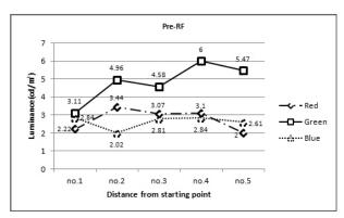
Figure 13. Effect of the luminance values by the color of light source in the condition of Pre-RF(unit: cd/m³) Pre-RF(Pre-etching × Reflective Fabric)
