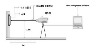
Figure 6. Method of luminance measurement
