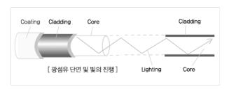
Figure 1. The principle of optical fiber CHARM LIGHTING. All Right Reserved.
