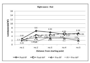
Figure 8. Effect of the luminance values by methods of weaving when the red light source(unit: cd/m²)
