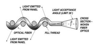
Figure 3. The mechanism of refraction in flexible POF LUMITEX. All Right Reserved.
