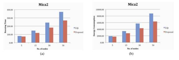
Fig. 2. Performance of the proposed scheme with respect to Z. Qi's Scheme (a) Running Time (s), (b) Energy Consumption (mJ).
