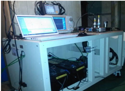
[Fig. 3] Energy saving unit of a hydraulic elevator
