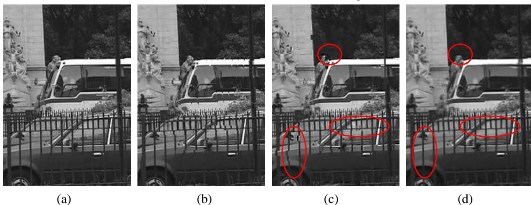
Fig.8. Results of SI extrapolation for Bus (18th frame). (a) Original; (b) MCE, PSNR = 20.19 dB; (c) AR_Fusion, R = 1 , PSNR = 24.58 dB; (d) MAAR_avg, R = 1 , PSNR = 25.83 dB.
