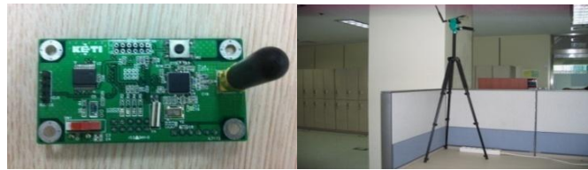
Fig. 10. CSS ranging hardware and installed AN
