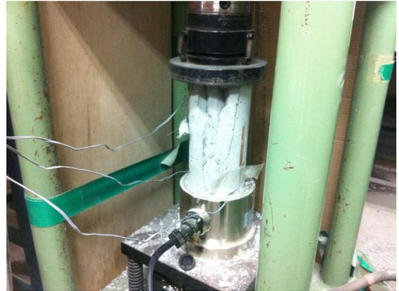
Fig. 5. Fractured specimen during uniaxial compression test
