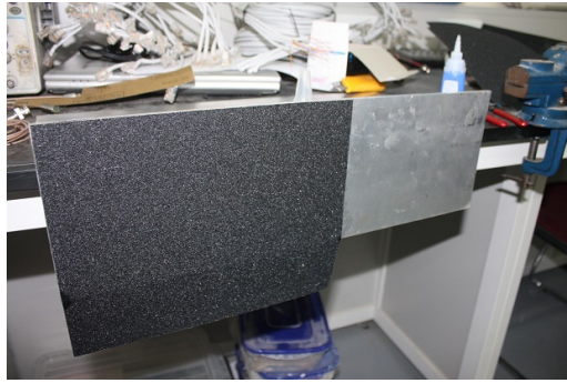
(a) Attach the sand paper on the wall base
