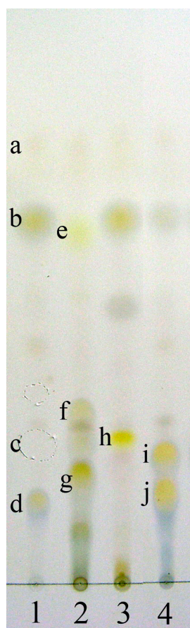
Fig. 2. Thin layer chromatography profile of Hypotrachyna species in solvent system A. 1, H. nodakensis with chloroatranrin (a), atranorin (b), protolichesterinic acid (c), gyrophoric acid (d); 2, H. osseoalba with lichexanthone (e), lividic acid (f), physodic acid (g); 3, Control [ Lethariella cladonioides (Nyl.) Krog] with norstictic acid (h); 4, H. revoluta with unknown 1 (i) and gyrophoric acid (j).
