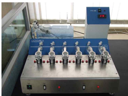
Fig. 2. Schematic Diagram of Transdermal Absorption Apparatus of Chemicals Release In Vitro .
