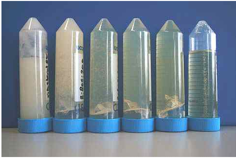
Fig. 4. Mixtures of 8% \beta -sitosterol+ \gamma -oryzanol in sunflower oil in various sterol(ester) ratios. The \beta -sitosterol: \gamma -oryzanol ratio from left to right: 100:0; 80:20; 60:40; 40:60; 20:80; 0:100. Both single sterol(ester) systems in sunflower oil are liquid, the binary sterol(ester) systems in sunflower oil are gelled. The firm gelled samples were scooped near to the cap, leaving a distinct fracture pattern (taken from ref 15).
