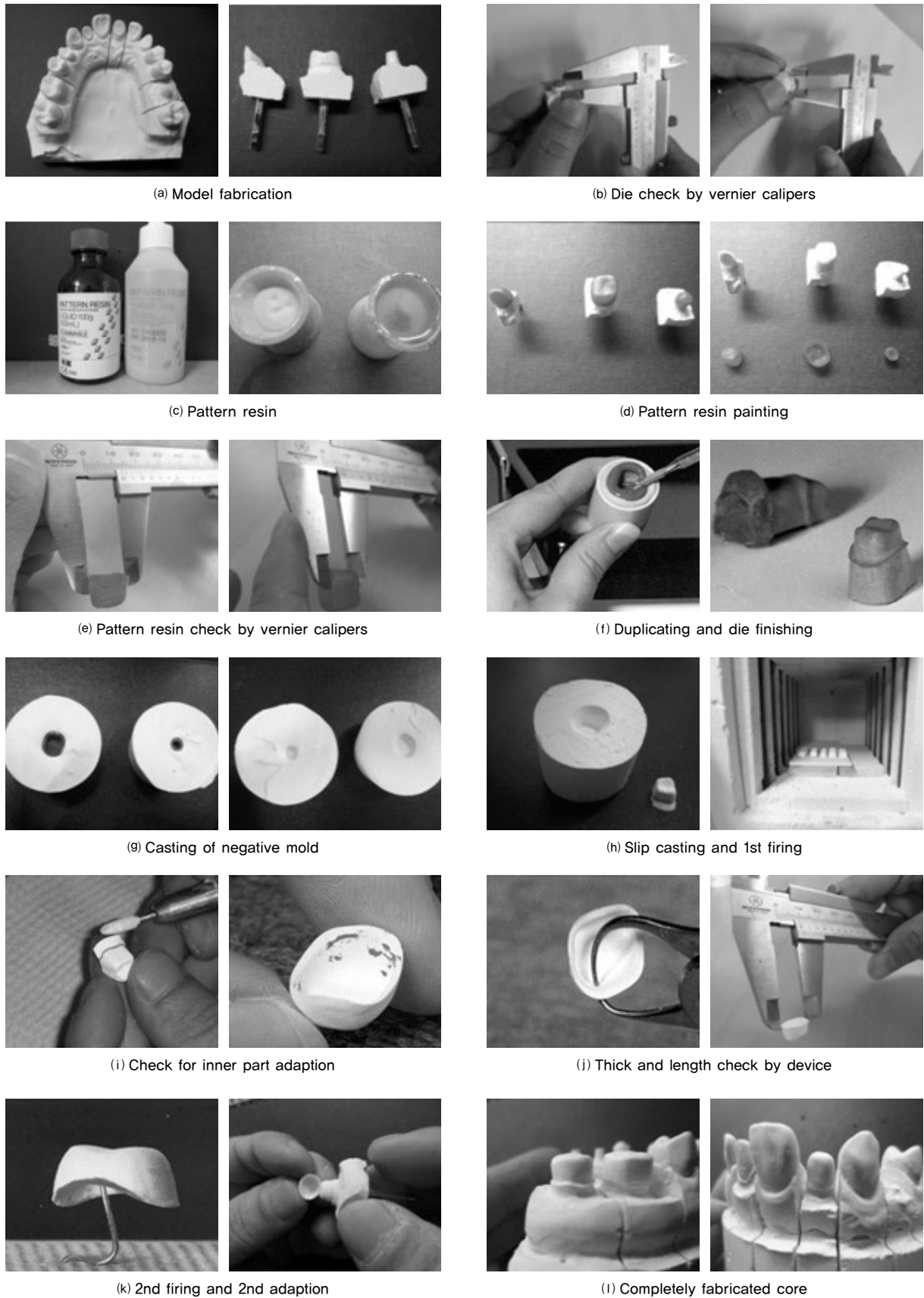
Fig. 2. Photographs of core manufacturing process
