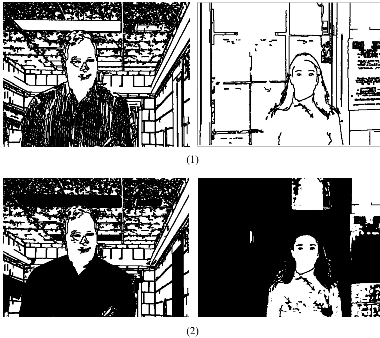
Fig. 7. Segmentation using edge and skin: (1) Canny edge with manual thresholds, (2) edge and skin segmentation results with separated face and background regions
