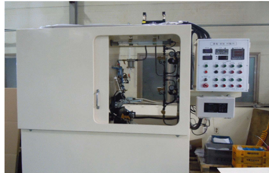
Fig. 4. Performance tester for low pressure fuel pump.
