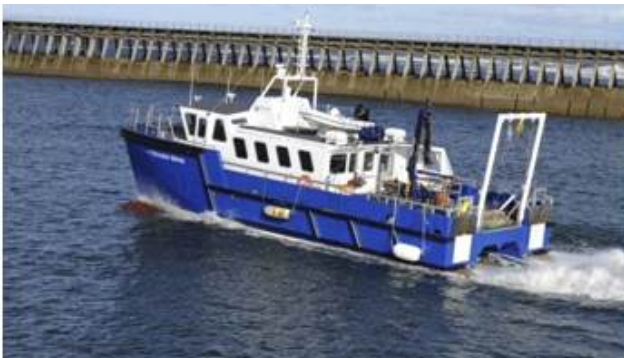
Fig. 1 Sea trial at design speed (15 knots)
