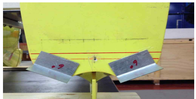
Fig. 3 Photo of 9 degree Trim Tabs mounted at the transom of the model
