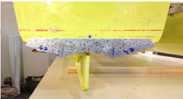
Fig. 5 Photo of Interceptors fitted to the model
