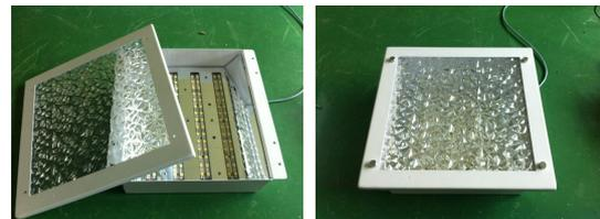
Fig. 12 Manufactured light diffuser
